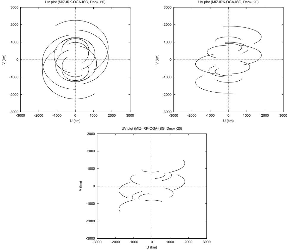
Figure 2:  $UV$  coverage ( $\pm 3000$  km) expected with VERA four antennas from an observation over elevation of  $20^\circ$ . Each panel show  $UV$  coverage for the declination of  $60^\circ$  (top left),  $20^\circ$  (top right), and  $-20^\circ$  (bottom).
