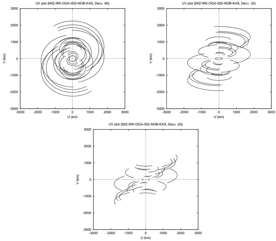
Figure 14:  $UV$  coverage expected with the array of the six antennas, VERA four antennas, NRO 45-m, and NICT 34-m telescopes, from an observation over elevation of  $20^\circ$ . Each panel show  $UV$  coverage for the declination of  $60^\circ$  (*top left*),  $20^\circ$  (*top right*), and  $-20^\circ$  (*bottom*).
