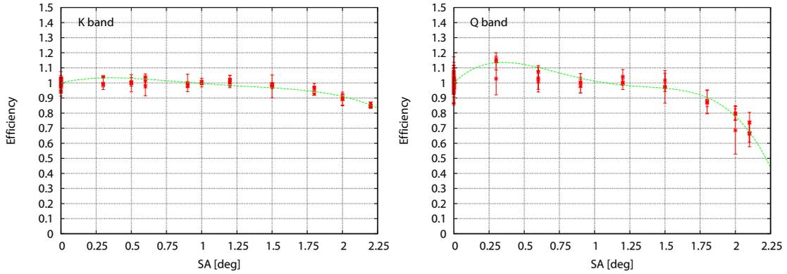
Figure 5: The dependence of the aperture efficiency on the separation angle between dual-beams in the K band (on Mar 4, 2004; *right*) and the Q band (on Mar 5, 2004; *left*) for Iriki antenna. The efficiency of vertical axis is relative value to the measurement at the separation angle of  $0^\circ$ . The curved line indicates the quartic polynomial fitting.
