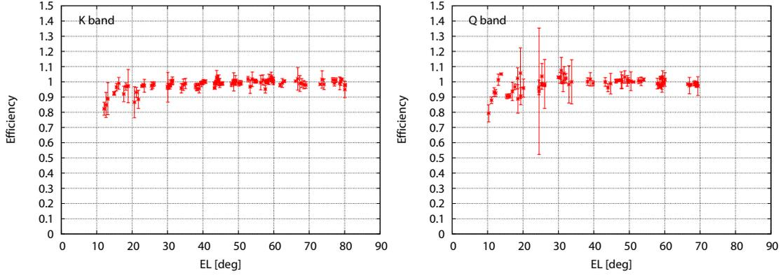
Figure 4: The elevation dependence of the aperture efficiency in the K band (on Feb 8, 2005; *right*) and the Q band (on Feb 12, 2005; *left*) for Iriki antenna. The efficiency is relative value to the measurement at  $EL = 50^\circ$ .
